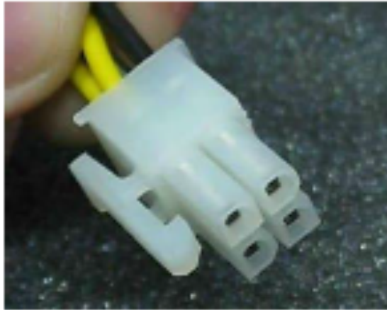
Conector macho ATX P2 de 4 pines
