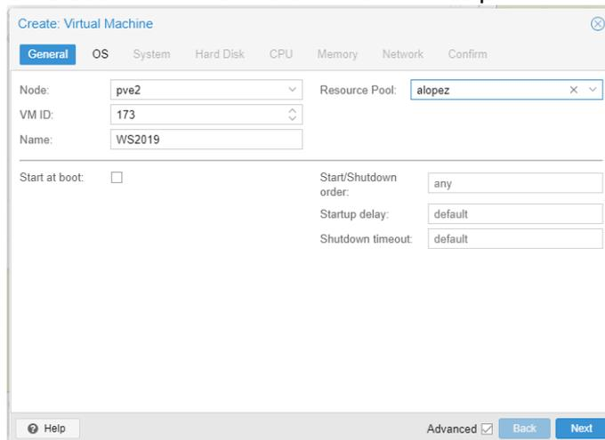
The screenshot shows the 'Create: Virtual Machine' dialog box in Proxmox VE, with the 'General' tab selected. The dialog has several tabs: General, OS, System, Hard Disk, CPU, Memory, Network, and Confirm. The 'General' tab contains the following fields and options:
